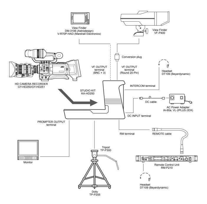
• Power is supplied by the Remote Control Unit RM-P210 via the 26 pin camera cable when in-use. If the Remote Control Unit RM-P210 is not in-use, use AC power adapter.
